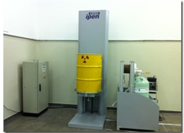
Figure 2. Automated system for isotopic characterization of radioactive waste drums.
